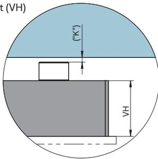
Dimension "K" required for heat expansion is to be ensured by grinding the pressure piece (12 + 0.1 mm)! Determine the difference between the height of the manifold system and the height of the frame plate when installed!  $\Delta T$  specifies the temperature differential between the processing temperature and the mould temperature!
