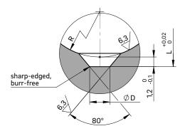
For open nozzles with a tip/open nozzles with a straight outlet for antechamber versions A/B and nozzle piece C
