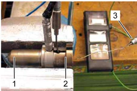
Fig. 49: Measuring position for external temperature measurement
