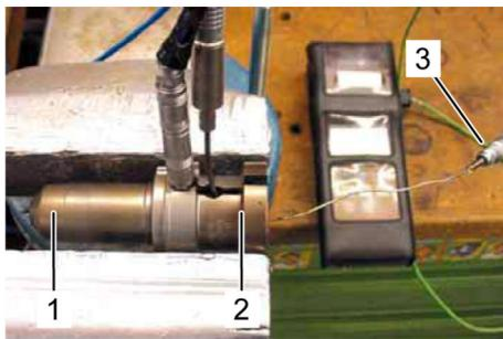
Fig. 48: Measuring position for external temperature measurement
