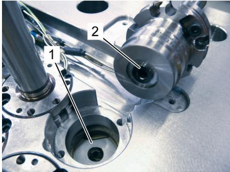
Fig. 16: Check the nozzle for leaks
