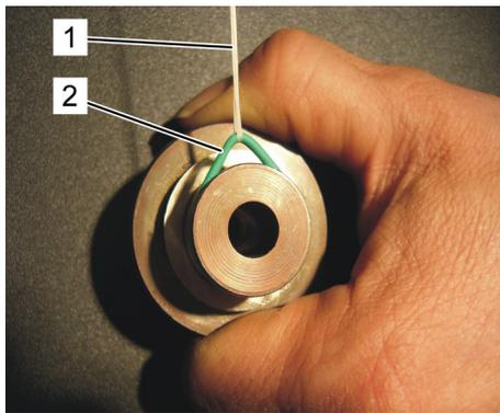
Fig. 57: Aligning O-rings
