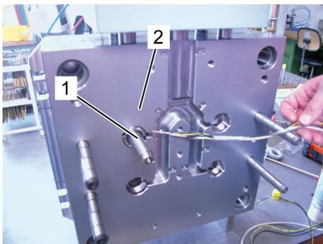
Fig. 65: Removing the nozzles
