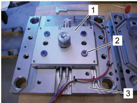
Fig. 17: Fitting the manifold and pressure pads
