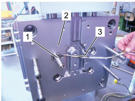
Fig. 18: Fitting the nozzles
