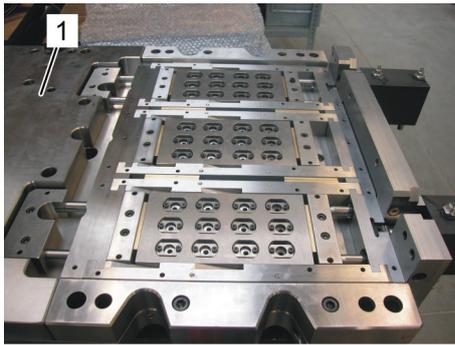
Fig. 26: Fitting the clamping plate
