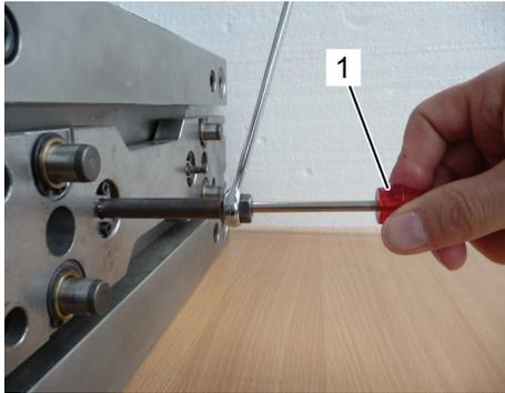
Fig. 33: Adjusting the needle
