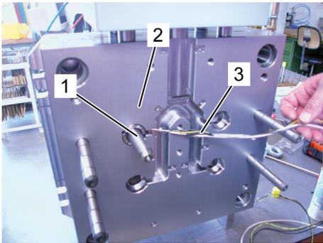
Fig. 15: Fitting the nozzles
