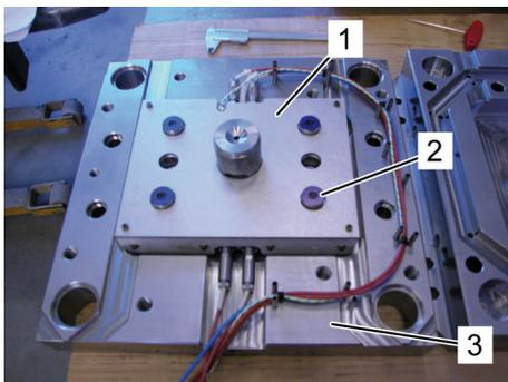
Fig. 66: Removing the pressure pads and manifold
