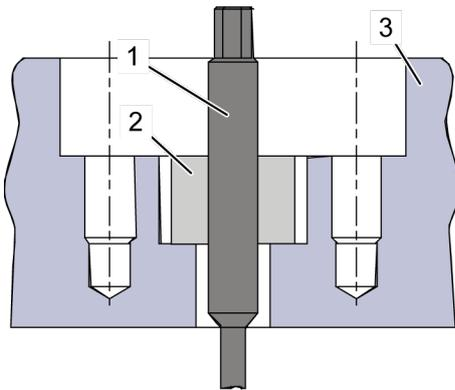
Fig. 29: Fitting the needle
