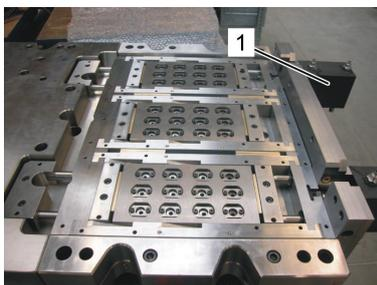
Fig. 28: Fitting the drive cylinder
