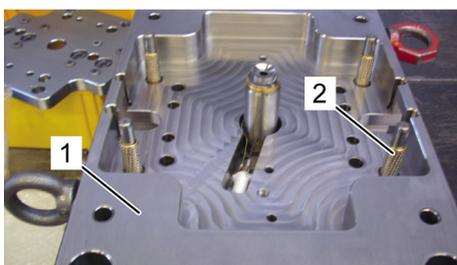
Fig. 24: Lifting plate
