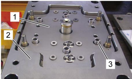
Fig. 25: Fitting the lifting plate mechanism
