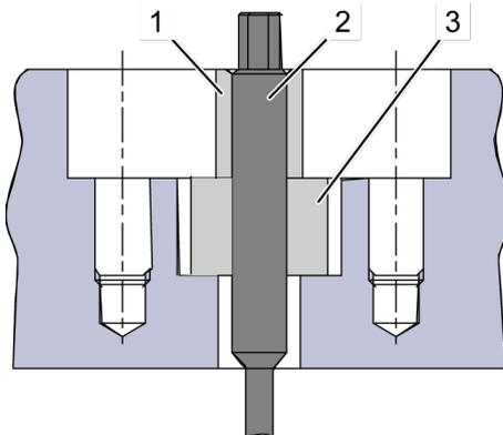
4. ➔ Remove the adjusting nut (1), needle (2) and piston (3) together using the auxiliary thread and hammer-action puller.
