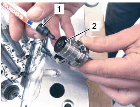
Fig. 13: Marking the sealing face on the nozzles
