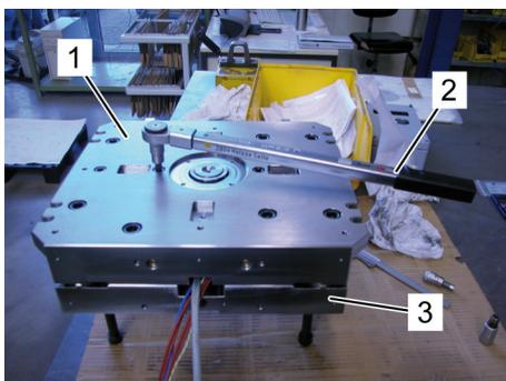
Fig. 14: Fitting the clamping plate
