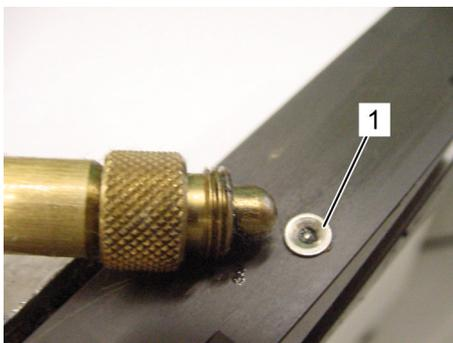
Fig. 59: Ball-valve impact hole
