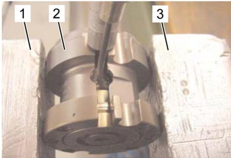
Fig. 41: Clamping the nozzle
