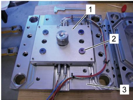
Fig. 12: Fitting the manifold and pressure pads
