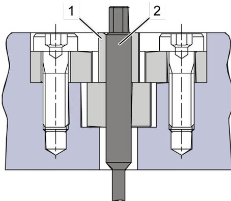
Fig. 60: Undoing the adjusting nut
