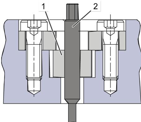
Fig. 31: Screwing on the adjusting nut
