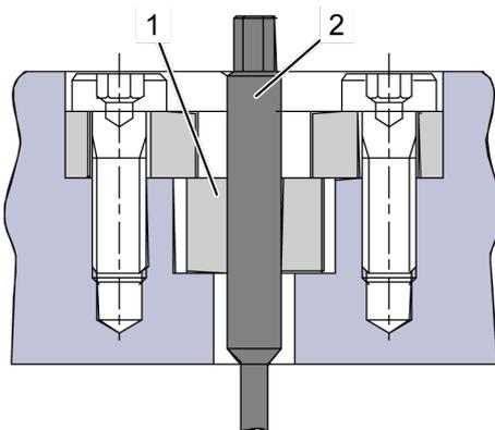
Fig. 61: Unscrewing the needle
