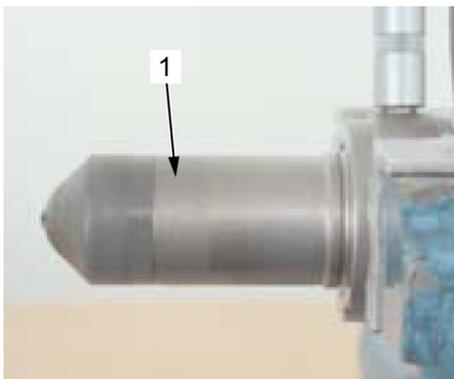
Fig. 42: Cross-section reduction
