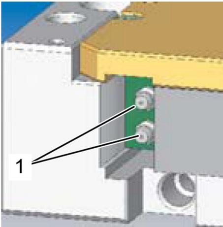
Fig. 58: Re-lubricating the sliding cam mechanism
