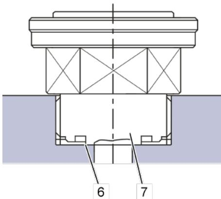
Fig. 55: Connection element
