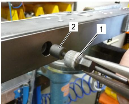
Fig. 51: Removing plugs
