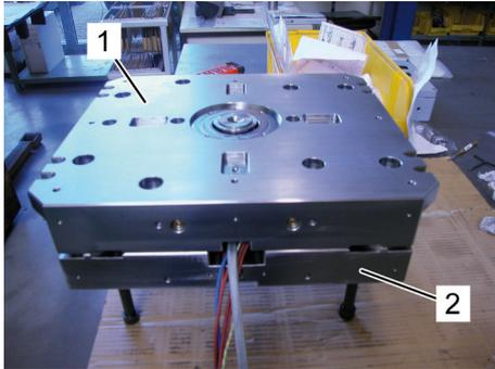
Fig. 64: Removing the clamping plate
