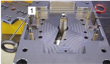
*Fig. 7: Example of ring screws as attachment points*
