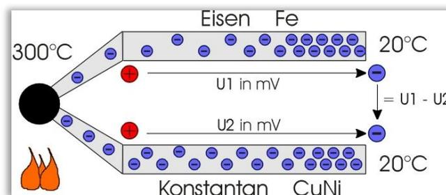
Figure 3: Thermocouple made of iron - constantan (FeCuNi)
